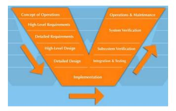
Figure 2: Typical Systems Engineering Process "V" Diagram
