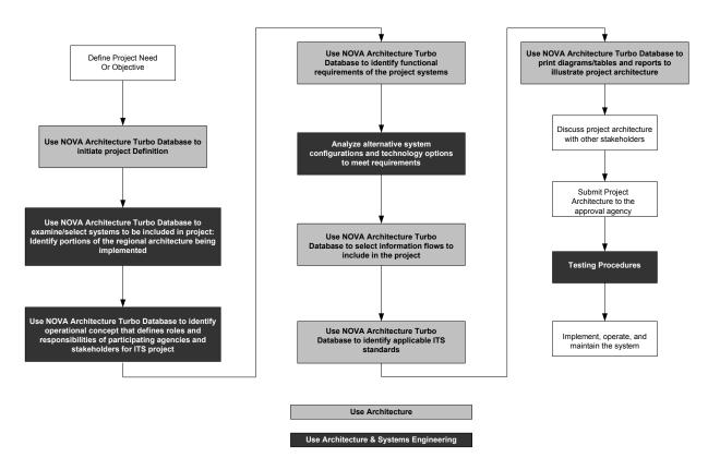
Figure 3: Process to develop Detailed Project Architecture (After Funding Approval)
