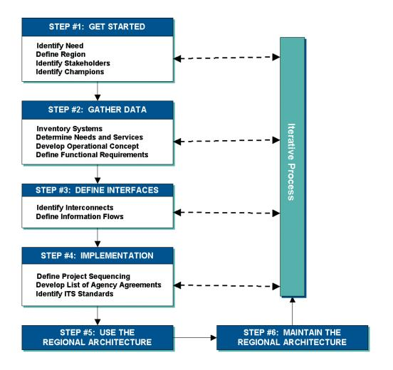
Figure 3. NOVA ITS Architecture Development Process
