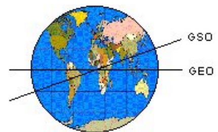
Figure 25 – Geostationary and Geosynchronous Orbits
